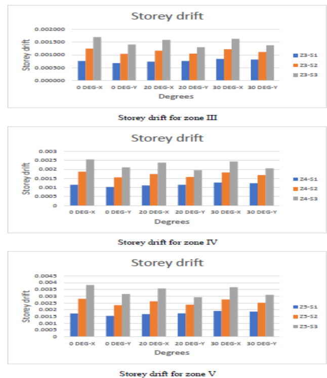
Chart -4: Storey Drift for 0°, 20° & 30° sloped ground building at storey level 4
